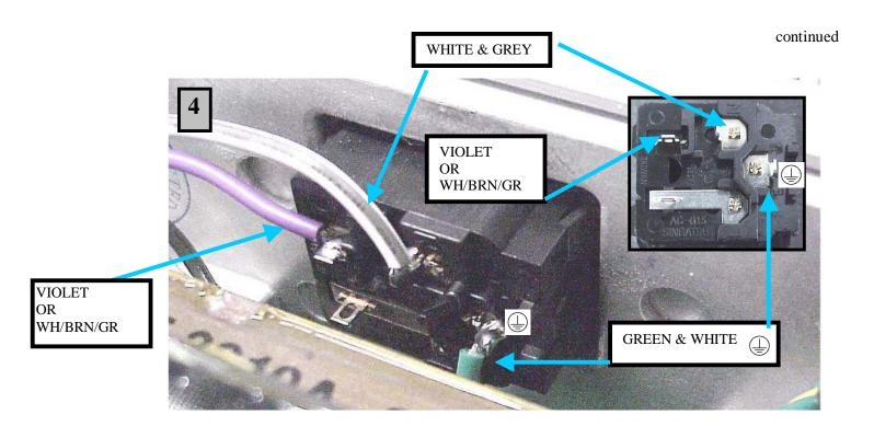
**REPLACE MODULE** with P/N 5065-6978. Before soldering perform "TEST FOR LOOSE AC MODULE" as shown in picture above. This will confirm that the new Module is secure. Solder wires and **REPLACE FUSE**.
